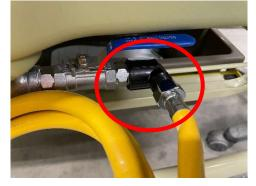
The extension is meant to be a permanent fixture of the drain assembly.
